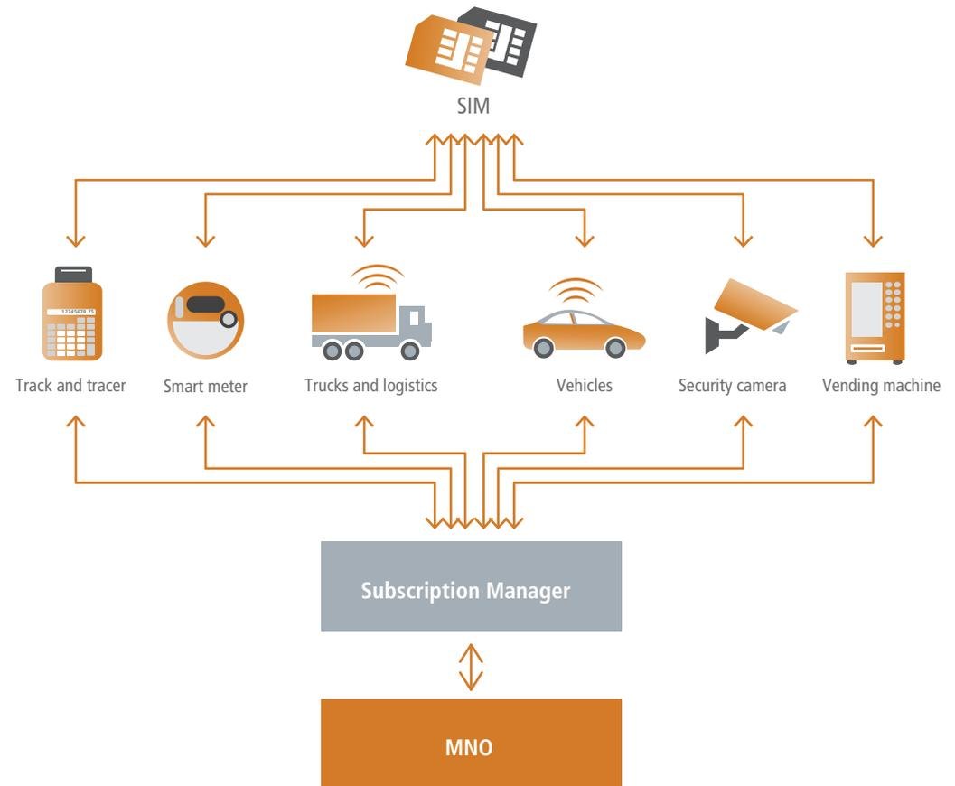
**Figure 14: Remote Provisioned SIM: Elements**
