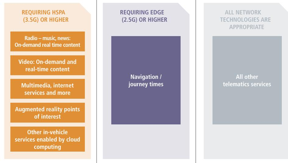
**Figure 37: Classification of Telematics and Infotainment Services by Bandwidth and Latency Requirements**
