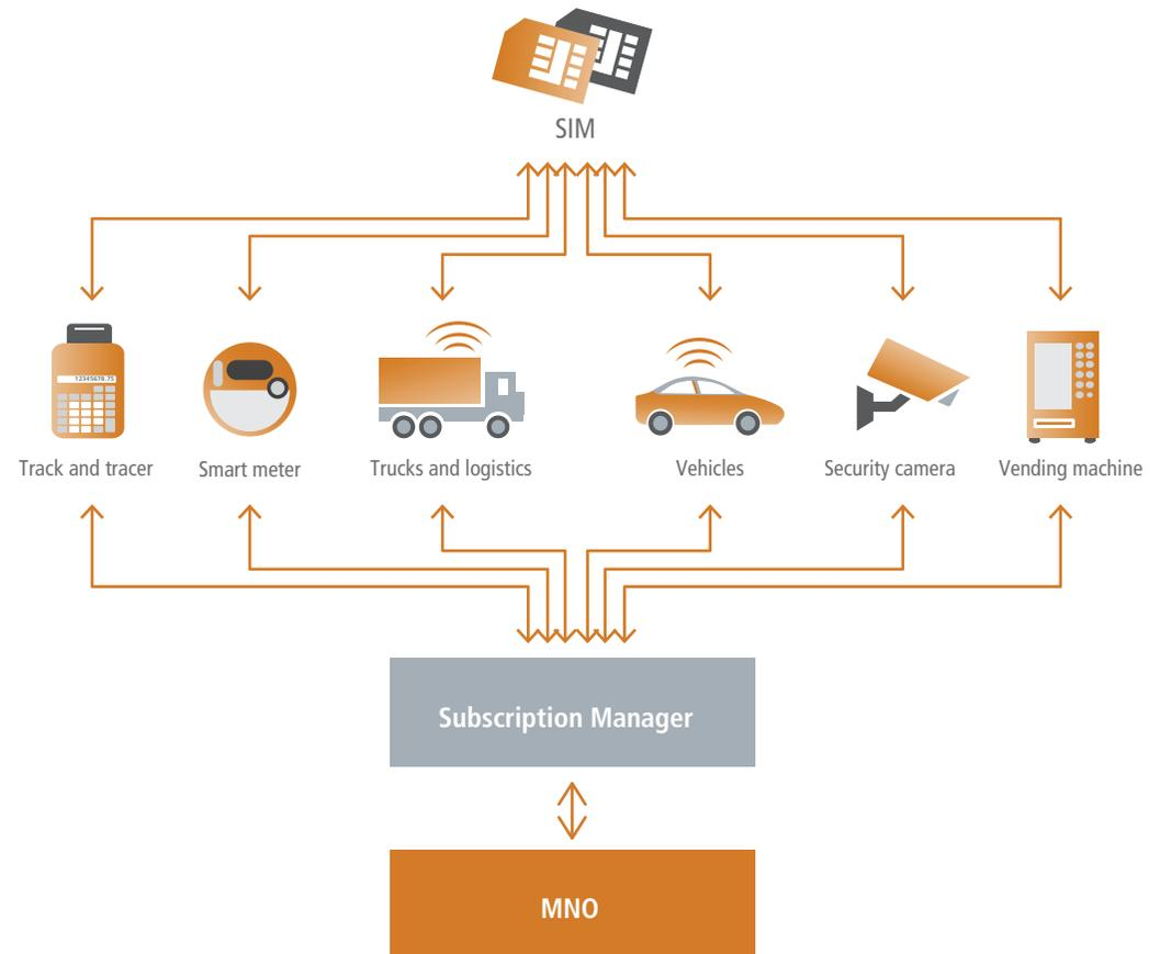
**Figure 14: Remote Provisioned SIM: Elements**
