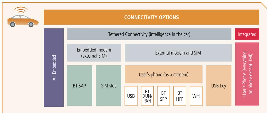
Figure 21: Different Means to Enable Car Connectivity: Source: SBD 2011
